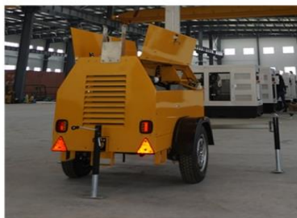
Integrated Road Signal Lights
